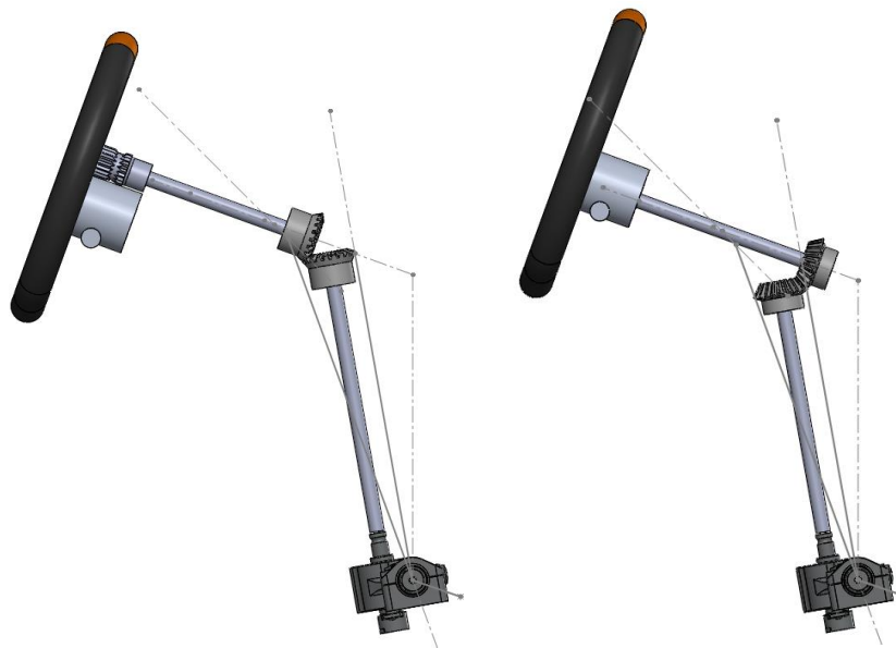
Figure 11: SolidWorks model of my two-steering gearbox, left side angle was 60^\circ . Right picture is 120^\circ gear angle
